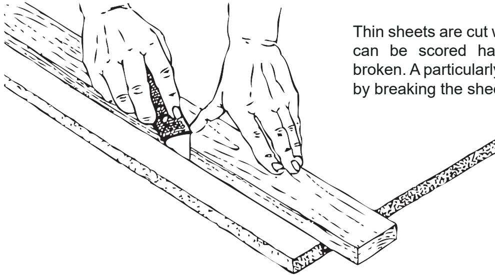
Thin sheets are cut with a knife. Thicker sheets can be scored half-way through and then broken. A particularly clean fracture is obtained by breaking the sheet at the edge of a table.
