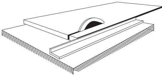
Circular saws are used for cutting sheets to size. Band and compass saws can be used for cutting shapes.
