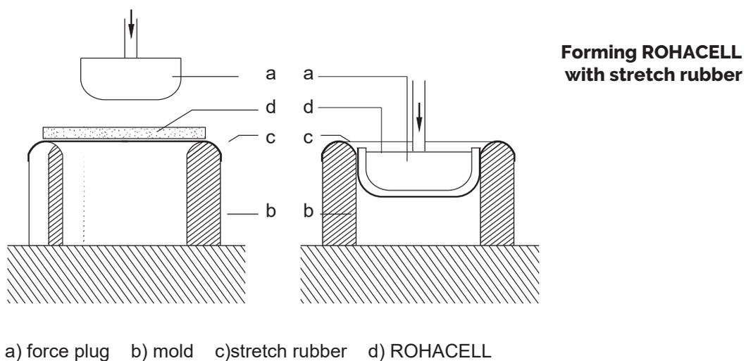
In order to ensure that the ROHACELL sheet can be drawn into the mold without much resistance, the edges should have large radii. If the radii are too small, the edge is squeezed into the heated foam at the start of forming and impedes further sliding. Cracks at these points will then be unavoidable. Forming itself should be done uniformly and quickly. Abrupt forming must be avoided.
